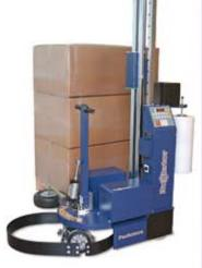
Automatic wrapping Robot for great quantities of pallet and suitable to work with high prestretch ratio. Easy to use, reliable, sturdy and without maintenance. Control panel created for any wrapping demand with personalizable programs. Available with or without power prestretch.
