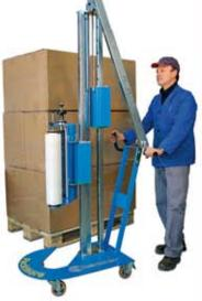
The most economic machine on the market. Wraps every kind of pallet. Very easy to use, without maintenance. The only system for packing at a distance of only 60 cm from the pallet. On this machine, the reel is lifted by a handle. Available with or without power prestretch.
